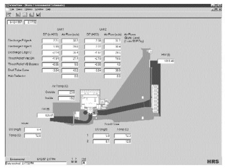
The WaterView software system, developed by Hydro Resource Solutions LLC (a partnership of Voith Hydro and the Tennessee Valley Authority), displays and analyzes environmental and operating parameters simultaneously. Using these data, the software determines optimal turbine settings to achieve environmental and generation targets, and supplies the information to the plant control system.
