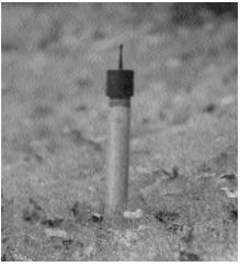
**Dataloggers for Small Hydro** The Mountain Energy 100 series dataloggers are designed for simplicity of use, durability, and reliability in the field. In this photograph, the downhole version of the logger, equipped with a radio data transmitter, is installed in a well at the 5-MW Big Creek project.
