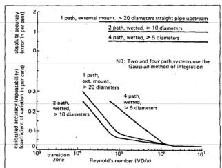
Fig. 1. Performance capabilities of the Westinghouse Leading Edge Flowmeter (LEFM). For absolute accuracy the determining factors are: pipe dimensions; upstream hydraulic configuration; integration technique; number of paths; and, Reynold's number. The determining factors for repeatability are: upstream hydraulic configuration; integration technique; number of paths; and, Reynold's number.
