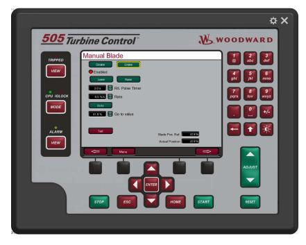
Figure 4-14. Manual Blade Screen
