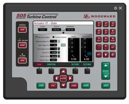
Figure 4-76 Actuator Outputs Screen
