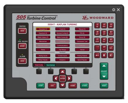
Figure 1-1. 505 Keypad and Display
