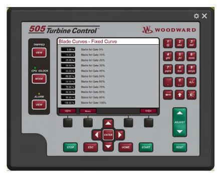
Figure 4-44. Blade Curves – Fixed Curve Screen
