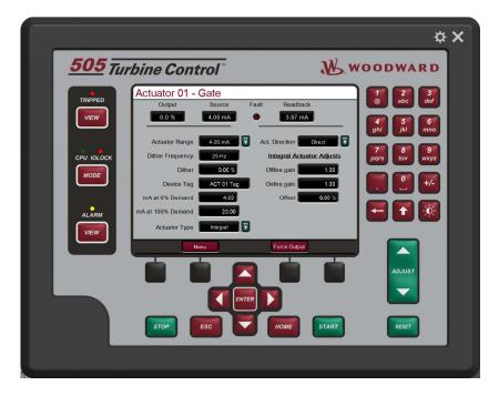
Figure 4-75. Actuator Output Screen
